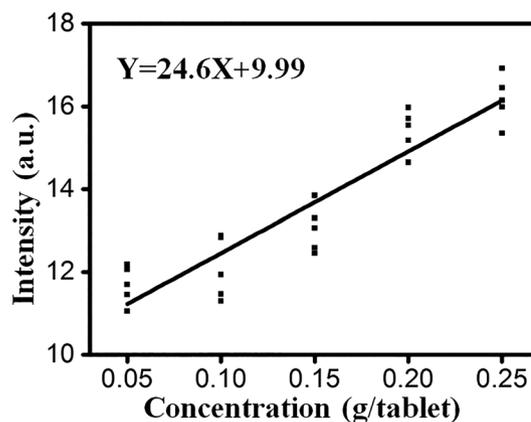
**FIGURE 5** Analytical curve of oxytetracycline based on simulated tablets using MALDI-MSI
