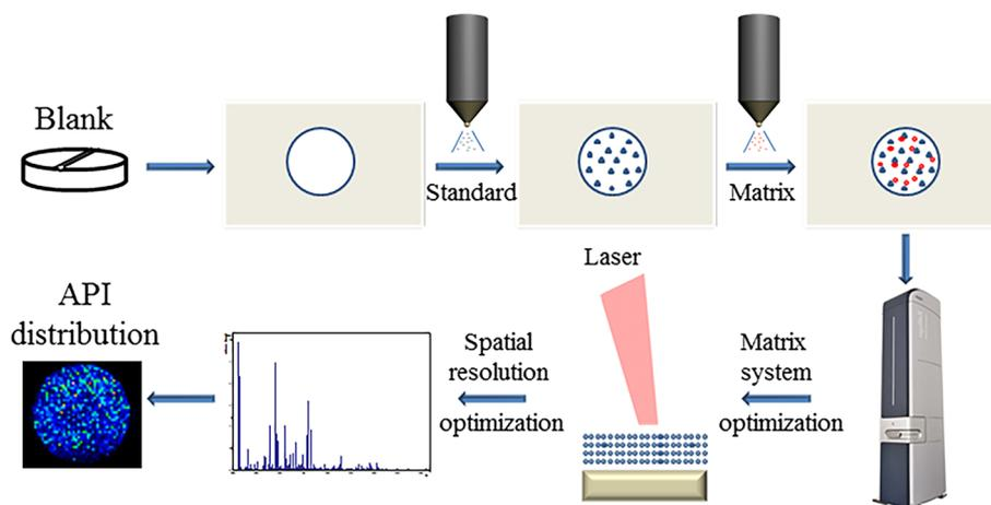
**FIGURE 1** Scheme of MALDI-MSI workflow for tablet analysis [Color figure can be viewed at [wileyonlinelibrary.com](http://wileyonlinelibrary.com)]
