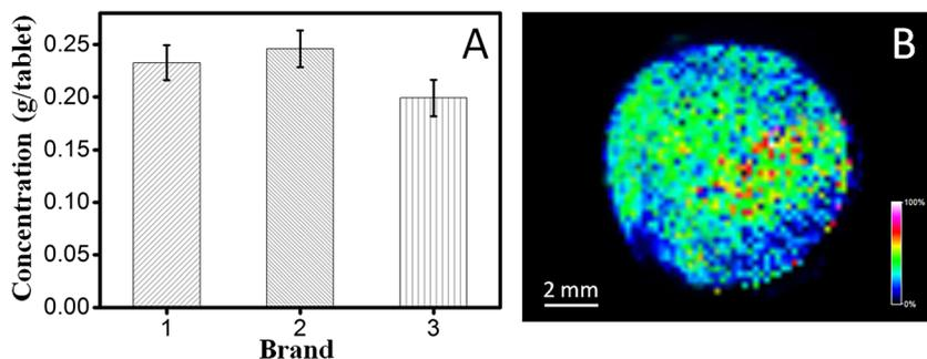
**FIGURE 6** A, Content of oxytetracycline in commercial tablets from different brands and B, MALDI-MS image of brand 3 sample at  $m/z$  461 ( $[M+H]^+$ ) [Color figure can be viewed at [wileyonlinelibrary.com](http://wileyonlinelibrary.com)]
