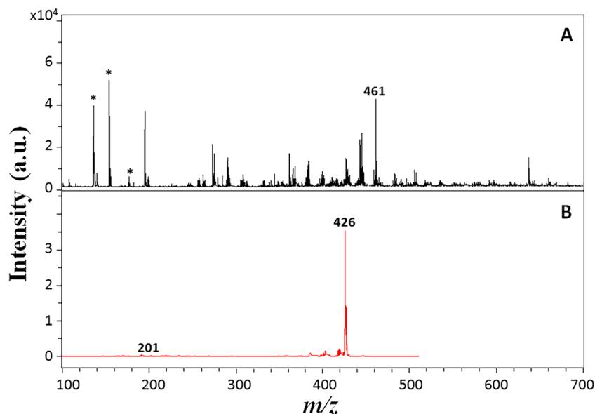
**FIGURE 2** A, Positive ion MALDI MS spectrum of oxytetracycline tablet using DHB matrix. The peaks for DHB ( $[M + H - H_2O]^+$  at  $m/z$  137.24,  $[M + H]^+$  at  $m/z$  155.24 and  $[M + Na]^+$  at  $m/z$  177.26) are labelled with asterisks. B, MS/MS spectrum of protonated oxytetracycline at  $m/z$  461 [Color figure can be viewed at [wileyonlinelibrary.com](http://wileyonlinelibrary.com)]
