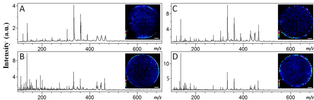
**FIGURE 4** Overall spectra and images at  $m/z$  461 of model tablet with different spatial resolution: A, raster at  $100\ \mu\text{m}$ , Smartbeam parameter: Single; B, raster at  $100\ \mu\text{m}$ , Smartbeam parameter: M5; C, raster at  $200\ \mu\text{m}$ , Smartbeam parameter: Single; D, raster at  $200\ \mu\text{m}$ , Smartbeam parameter: M5. The scale bar represents  $1\ \text{mm}$  [Color figure can be viewed at [wileyonlinelibrary.com](http://wileyonlinelibrary.com)]
